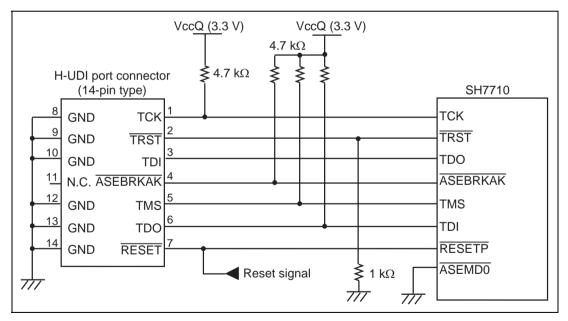
Figure 1.7 Recommended Circuit for Connection between the H-UDI Port Connector and MPU (14-Pin Type)
